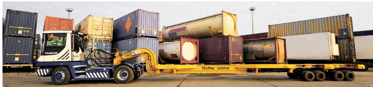
“The Liftec Cassette system offers improved safety, cost-effectiveness and high transport efficiency.”
