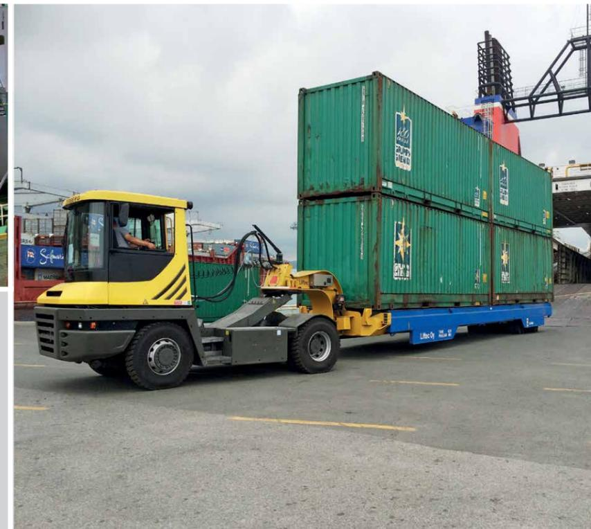
“The Liftec self-loading cassette system provides an effective and economical solution for RORO operators.”
